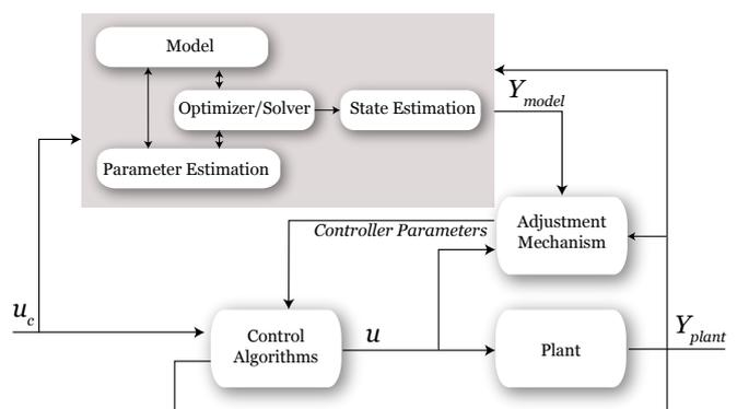
Figure 5: The model reads the inputs of the plant  $u_c$  and predicts the output  $Y_{model}$ . After comparison of its predictions with the actual outputs  $Y_{plant}$ , it subsequently adjusts its parameters for a more accurate estimation of the current plant state
