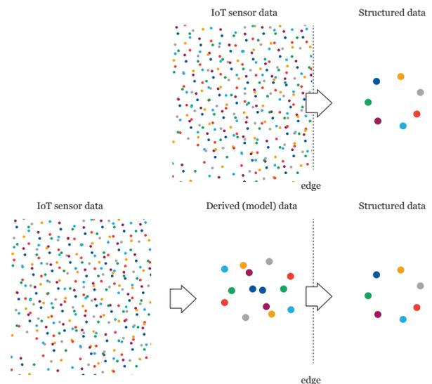
Figure 2: Performing analytics at the edge reduces storage, energy and bandwidth requirements
