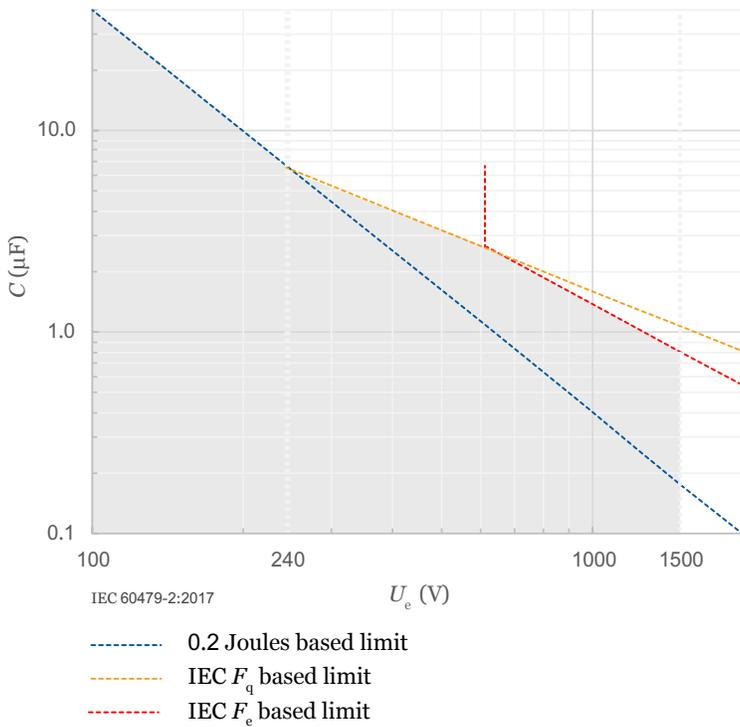
Figure 4: Capacitance limit vs Voltage. The blue line corresponds to the 0.2 Joules limit imposed by several standards. The range of applicability of the  $F_q$  based limit starts at 240 V.
